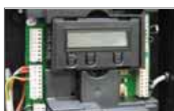
Control unit SEA 380 DG programmable on display
