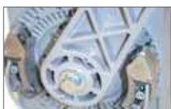
Adjustable mechanical and electronic limit switches in opening and closing
