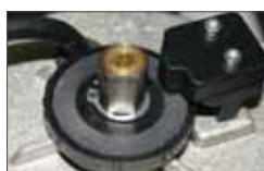
Mechanical twin-disk clutch
