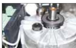
Electric motor and gears in oil lubrication
